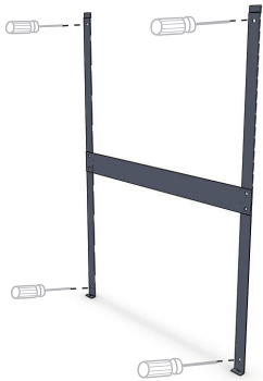
1. Screw H bracket to wall.
