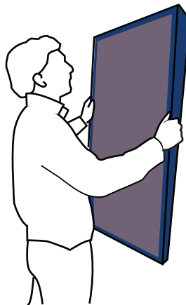
2. Place top of mirror frame over top tabs of H bracket.
